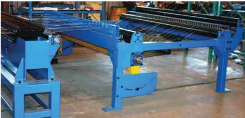
LBU SHOWING SPRING LOADED ARMS
