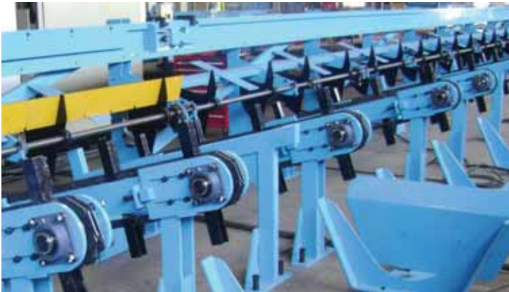
BUNDLE BATCHING STATION
