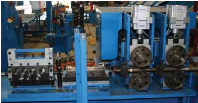
FEED ROLLS TO CROSS WIRE PLACEMENT
