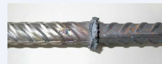
Flash butt welding of wire for reinforced concrete steel
