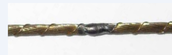
Welding of steel cord
