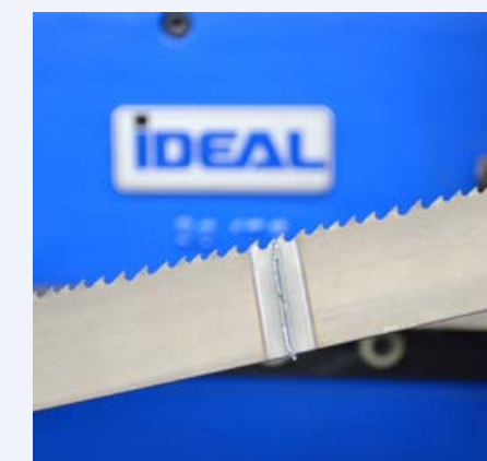
Weld seam, undeurred
