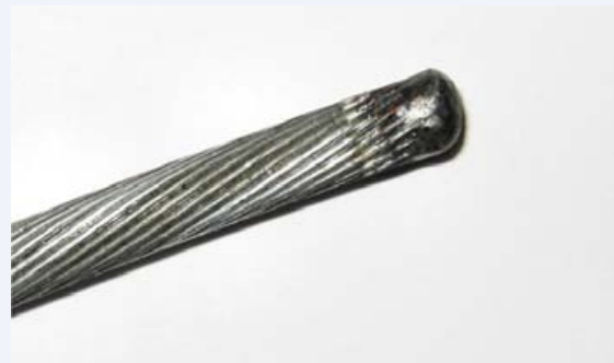
Separated, molten cable end
