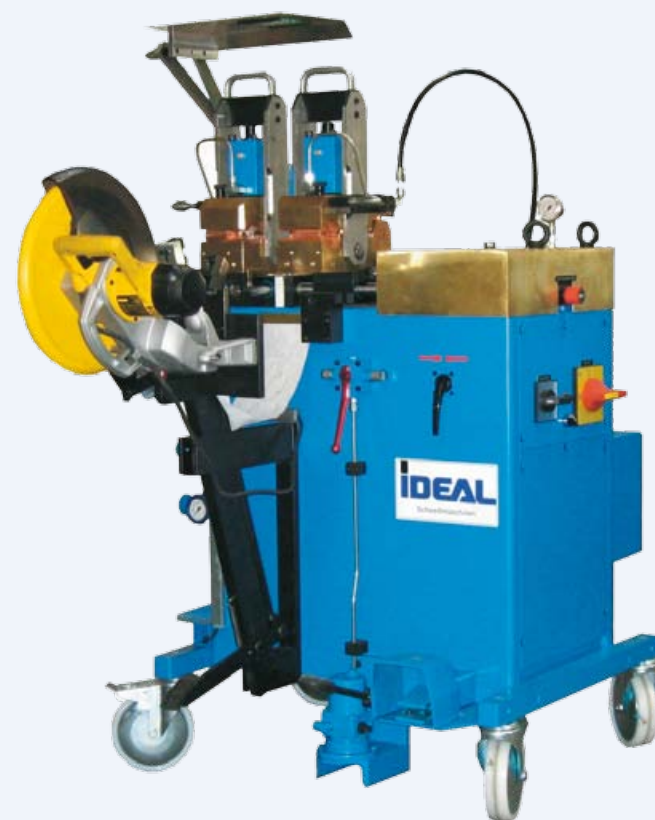
LSO 630 butt welder for stranded conductors
