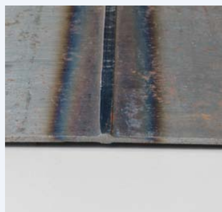
Flash butt welding, deburred
