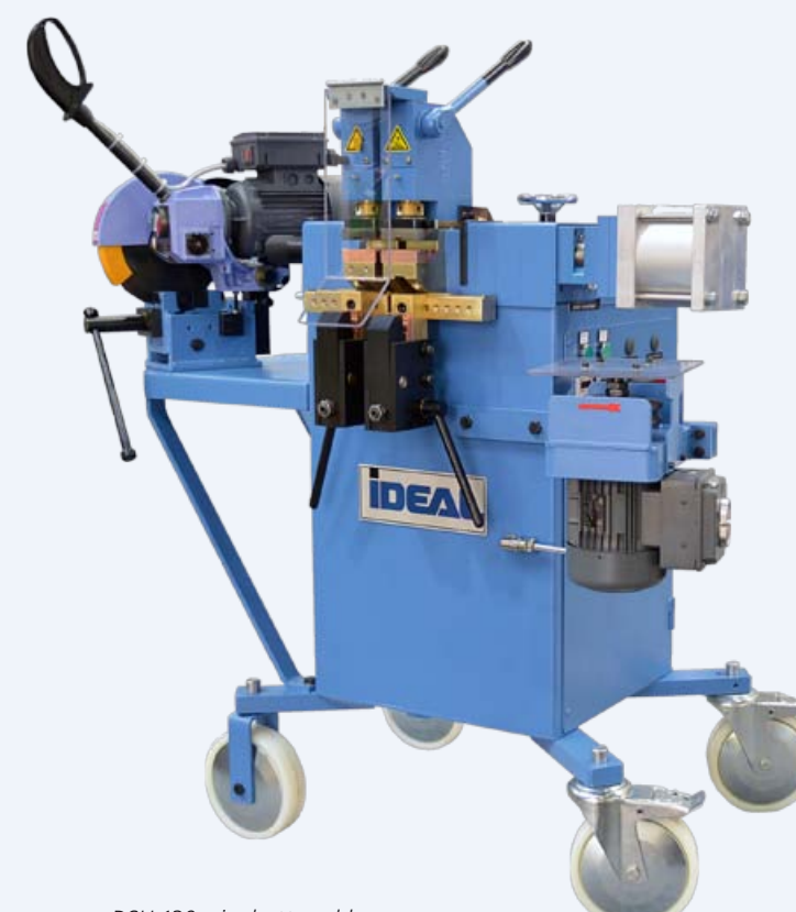
DSH 130 wire butt welder
