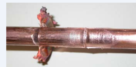
Dual force welding of copper wire
