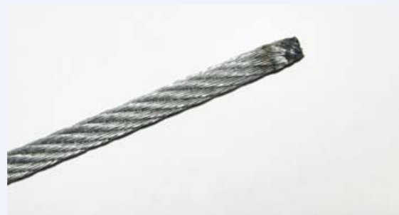
Tapered cable end-twisted during the separating procedure
