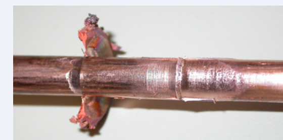
Dual force welding of copper wire
