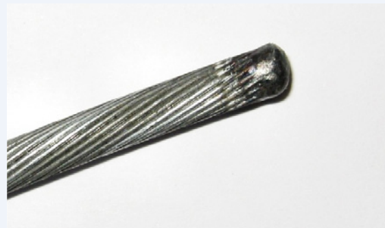
Separated, molten cable end
