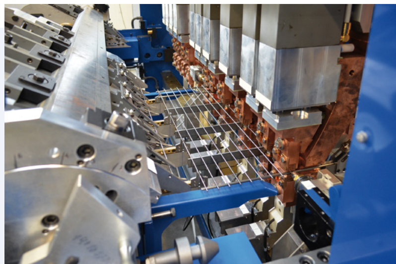
Cross wire magazine with flat bar mat
