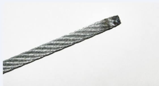
Tapered cable end-twisted during the separating procedure
